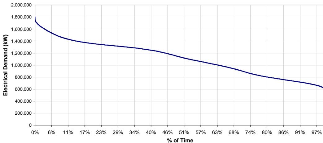
Figure 3 is a more detailed illustration of the peak 2003 loading periods for the Auckland/North-Isthmus region and which shows that the region peaked at 1,800 MW. This detailed load duration curve can be sliced into the following three areas that are indicative of the electrical energy that is consumed during peak times:
