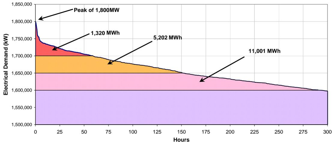
By way of illustration Figure 4 shows the half hourly periods and week days during which the regions load exceeded the 1,700 MW level during 2003. The months during which the periods occurred were July, August and September (i.e. a three month period). During this period the 1,700 MW level was exceeded on 33 days, with most periods occurring during the evenings and none occurring during weekends. The worst case consecutive period during which load exceeded 1,700 MW was for 4.5 hours.
