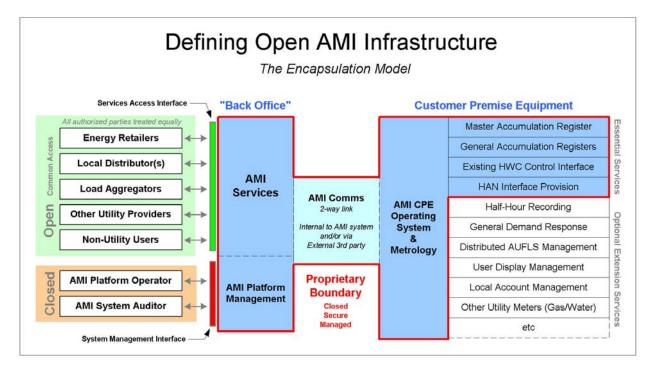
39. This diagram illustrates how open proprietary AMI systems could be deployed without creating a barrier to competition. Parties interested in offering services to end users across the system would contract for access via the "Services Access Interface" (shown in green). Distributors may be given preferred access to load control under special circumstances, such as if network security is threatened, but otherwise all parties using the platform services should be treated equally.
