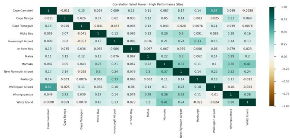
Figure 15 - Correlation between the selected wind sites. Note that the inter-regional correlation for wind is lower when compared to intra-regional values
