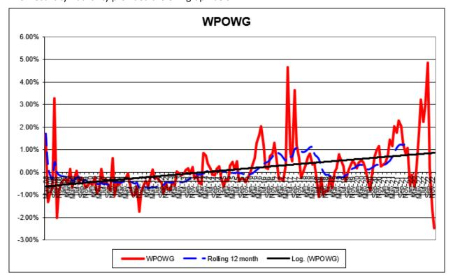
The UFE graph supplied by the Electricity Authority indicates that the 14-month UFE is tracking just above the accepted +/-1% threshold. As this is trending up above 1% it would suggest that further investigation is warranted to ensure Westpower's loss factors are accurate. I recommend that Westpower review the loss factors.
