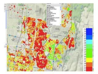
It shows significant points where the network voltage is above 255V, on a nominal 230/240V network.
