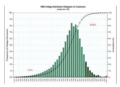
The significant information here is that the voltage is out of range for significant amounts of time – essentially non-compliant with supply regulations.
