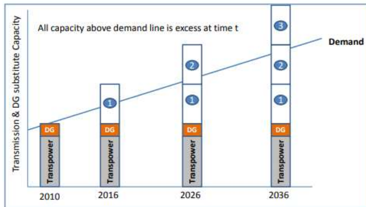
Figure B - Correct Economic Perspective: DG is part of in-use capacity, Transpower upgrade results in excess capacity (AIEG)
