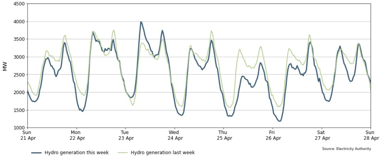
7.10. As a percentage of total generation, between 21-27 April, total weekly hydro generation was 55.1%, geothermal 20.3%, wind 11%, thermal 11.2%, and co-generation 2.4%, as shown in Figure 15. The relative decrease in hydro generation this week can be related to the relative increase in wind generation, as hydro operators seek to conserve water for winter.
