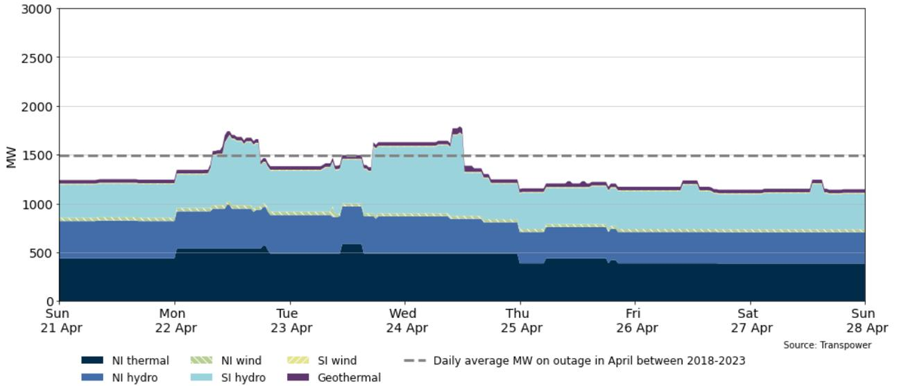
**Figure 17: MW loss from thermal outages between 21-27 April**
