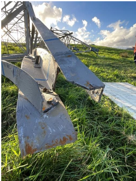
Photo A.23: Leg D of fallen tower. Ruptured from stub leg attached to foundation.
