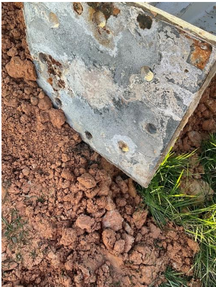
Photo A.19: Underside of baseplate of leg C. Some damage to the bolt hole closest to the ground (eastern side of base plate), which aligns with broken bolt.
