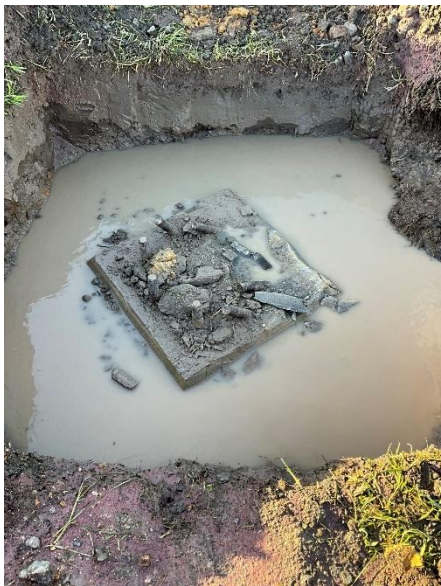
Photo A.8: Leg C foundation after being drained. No holding down bolts with nuts installed. Five holding down bolts on the eastern side bent towards the west, with the bolt furthest to the east broken in two places. No obvious evidence to suggest that the nuts had been stripped from any of the holding down bolts.
