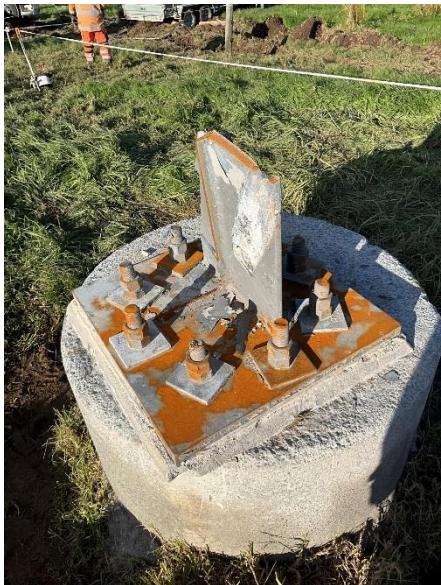
Photo A.12: Leg D ruptured. No nuts removed. Sign of sand blasting to base plate, bolts and nuts.
