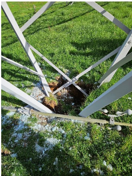
Photo B.13: Tower crossarm embedded in the ground from tower fall.
