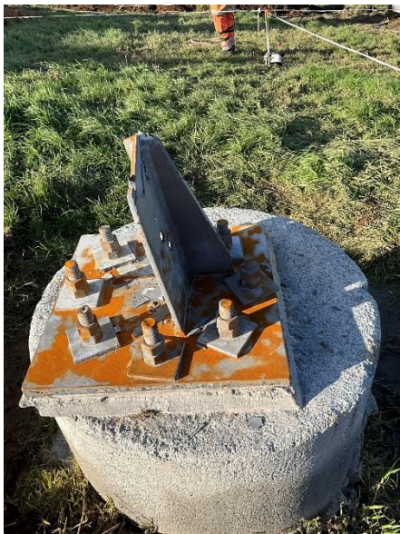
Photo A.13: Leg D ruptured. No nuts removed.
