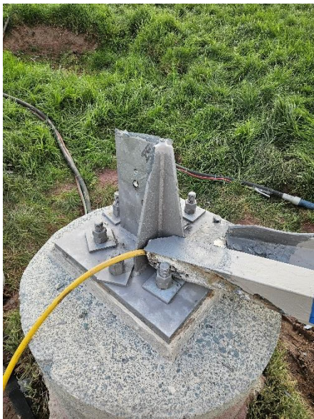
Photo B.10: Leg D ruptured leg and foundation.
