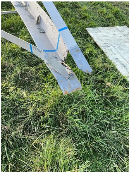
Photo A.22: Leg D of fallen tower. Ruptured from stub leg attached to foundation.
