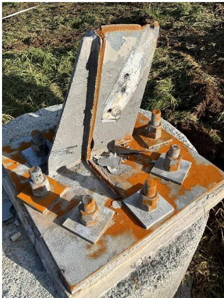
Photo A.15: Leg D ruptured. No nuts removed.
