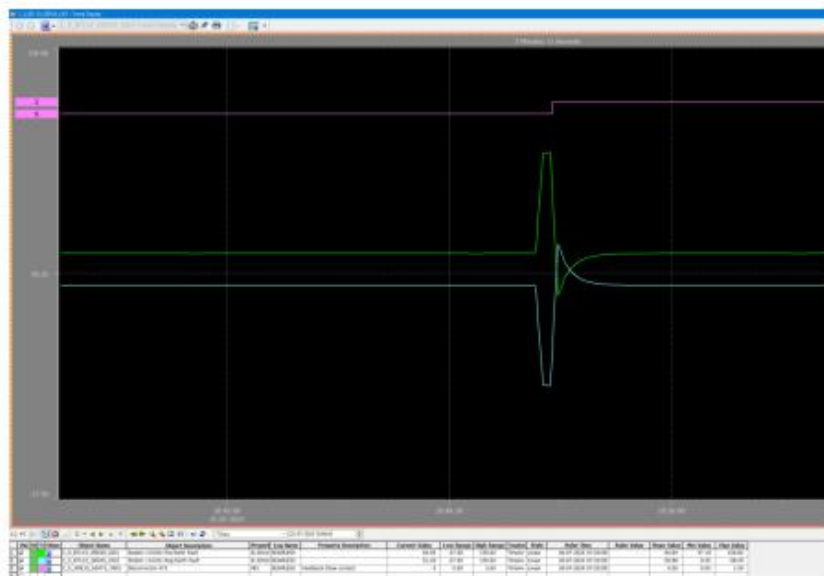
Figure 3 - CYD generating station DC traces during the earth fault
